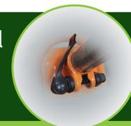
To tighten a quick release lever, push the handle inward so it makes a "V" shape with the bolt.
